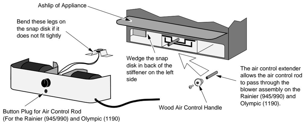
Make sure the wires leading to the snap disk are routed above the left side blower outlet (to prevent damage to the wires during installation). Install the blower following the directions below.
