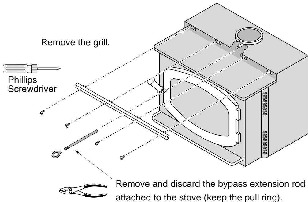
2. Install the top air chamber extension following the directions below.
