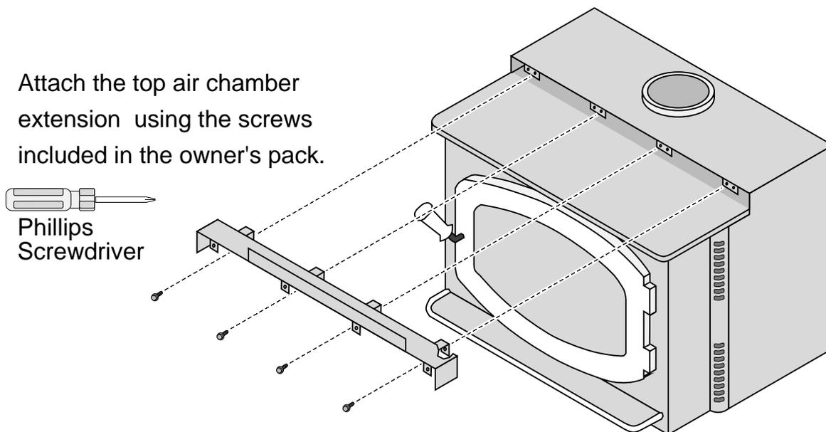
3. Attach the grill to the air chamber top. Attach the bypass extension rod included in the owner's kit to the damper yoke. Attach the bypass pull ring to the extension rod to complete the installation.
