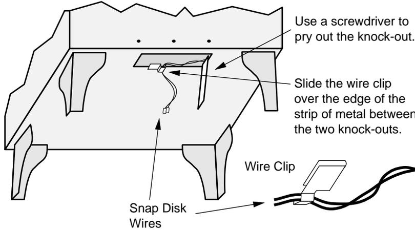
Feed the two snap disk wires into the eye of the wire clip. Remove all slack from the wire, making sure not to dislodge the snap disk. Pinch the eye of the wire clip to secure the wires.
