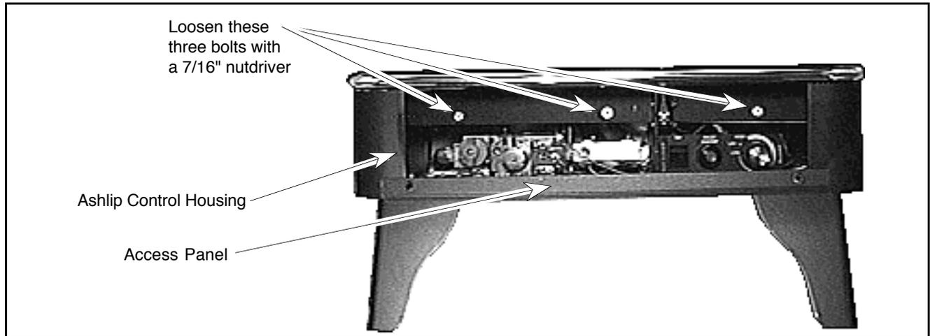
4. Disconnect the molex connector that attaches to the power cord. Remove the power cord from the heater by threading the molex plug through the hole in the ashlip control housing (see the illustration below). To route the power cord to the left side, follow step 5A. To route the cord to the rear (stoves only), follow step 5B.
