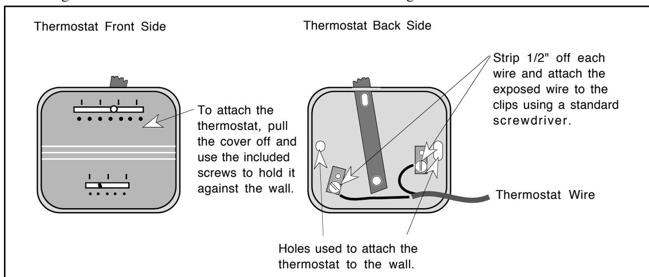
7. Remove the cover of the thermostat by pulling it apart carefully. The thermostat has mounting holes on each side of its base. Use the included screws to attach the thermostat to the wall. Tuck any excess wire behind the thermostat and replace the thermostat cover.
