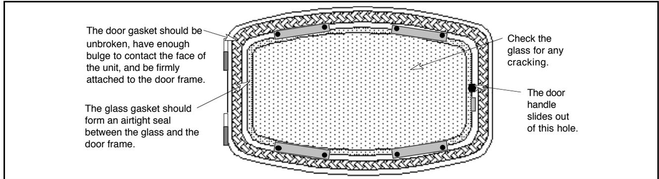
3. Then replace the door. Turn the door handle clockwise until the door seals tight. **Make sure the handle faces outwards and is not in front of the glass.**
