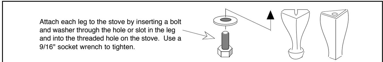
To level the stove, lift the stove up and unscrew each leveling bolt the appropriate amount. The rubber tips of the leveling bolts will tear if they are adjusted while weight is applied to them.
