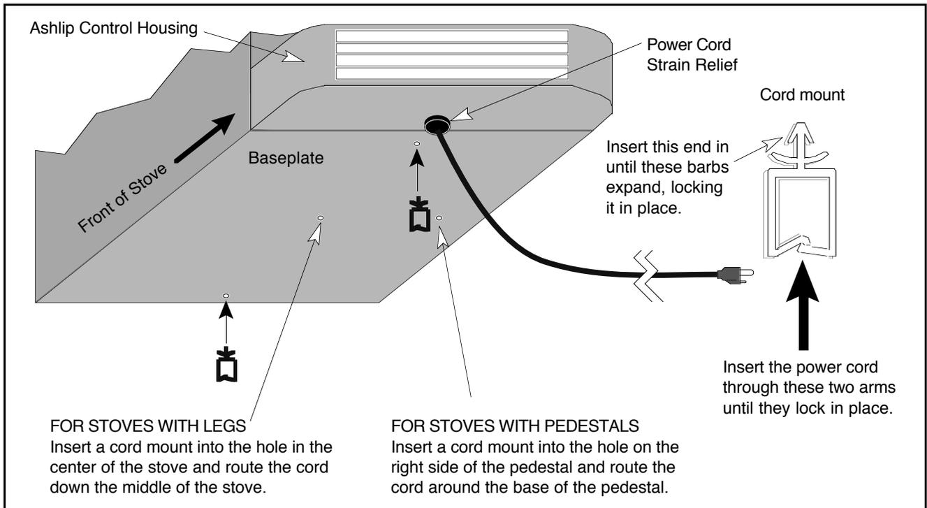
6. Replace the ashlip control housing, making sure no wiring becomes pinched, and tighten the three bolts that hold it in place.
