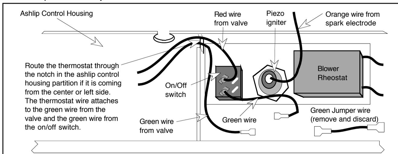
5. Replace the ashlip control housing. Make sure none of the wiring is pinched.
