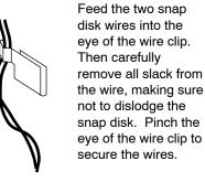
Secure the snap disk wires in place following the directions below.
