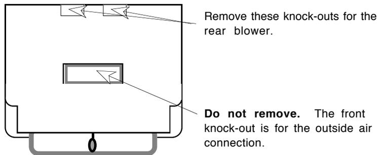
2. Feed the two wires coming from the thermodisk assembly through the stove and out the left side knock-out that was removed in step 1. Take the thermodisk assembly and insert it directly below the ashlip into the left side of the air intake. The thermodisk assembly should be positioned just behind the support tab that sits at an angle to the left front corner.
