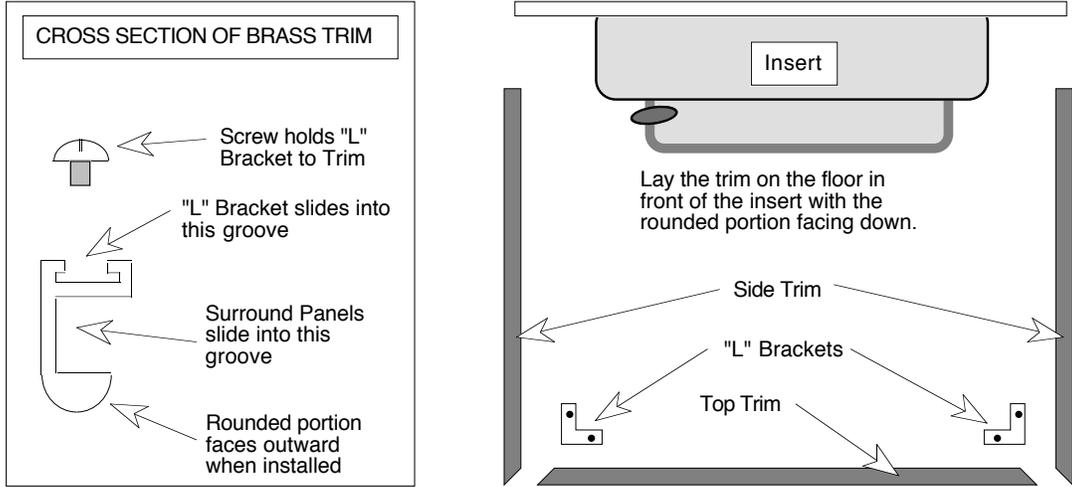
2. Insert an "L" bracket leg into the groove in the 45° cut end of each side piece. Slide the other leg of each "L" bracket into the groove in each end of the top piece.
