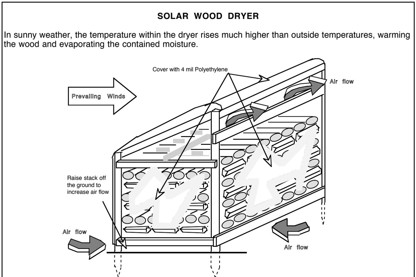
Many arrangements for plastic covering are possible. Thin 2 millimeter, clear polyethylene sheeting sold for drop cloths or garden mulching is not recommended because it is easily torn. The 4 millimeter thickness is more satisfactory and less costly than 6 millimeter. Any clear polyethylene deteriorates badly after a few months of exposure to full sunlight, so the stack may have to be re-roofed to remain dry over winter.
