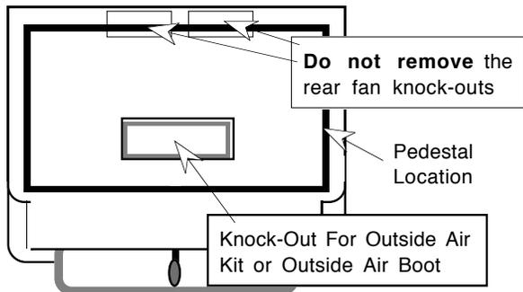
After the precise location of the stove is determined, the outside air kit or boot should be installed prior to installing the stove. Follow the directions included with the outside air kit or boot. Make sure to remove the correct knock-out for the outside air kit or boot. See the illustration to the left.
