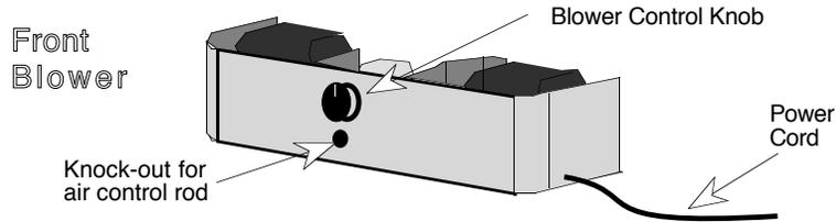
1. Remove the small knock-out located just below the blower control knob on the blower assembly (see the illustration above). Then remove the air control knob (located below the ashlip) by unscrewing it.
