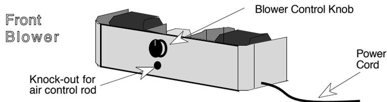
1. Remove the small knock-out located just below the blower control knob on the blower assembly (see the illustration above). Then remove the air control knob (located below the ashlip) by unscrewing it.
