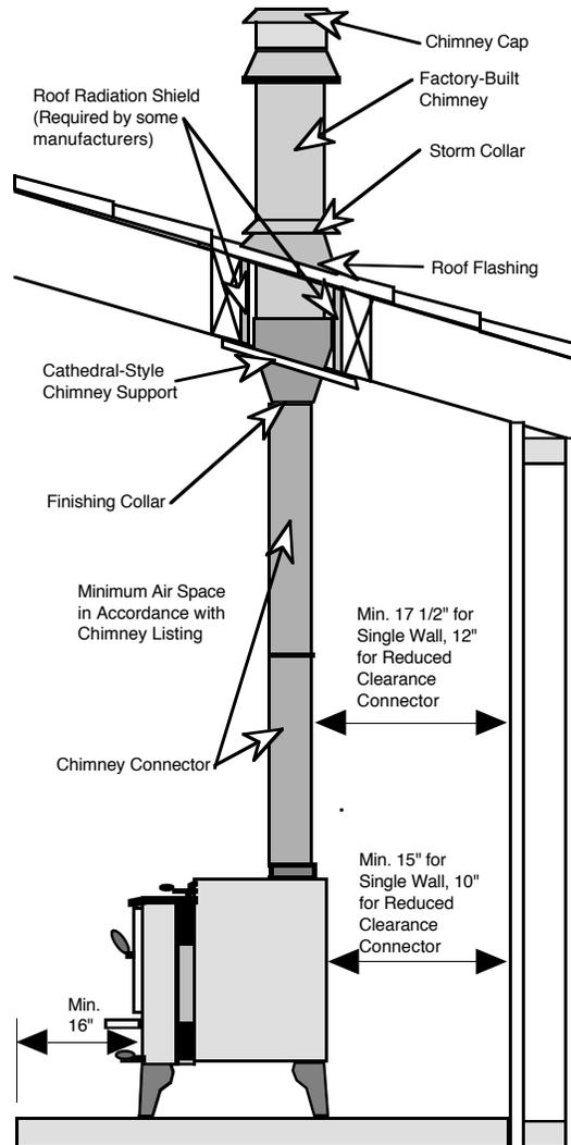
**IMPORTANT:** Because of the slope of the cathedral ceiling, care should be taken to extend the chimney sufficiently far into the room so that the chimney connector will meet the minimum clearances requirement from the sloped combustible ceiling. The greater the pitch of the ceiling, the further into the room the chimney section must extend. Use the concepts from "CHIMNEY INFORMATION & REGULATIONS" to accurately measure the appropriate distance from a sloping ceiling.
