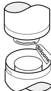
Apply a 1/8" bead of high-temperature silicone to the inner pipe. The silicone must seal the inner pipe from the outer pipe.
